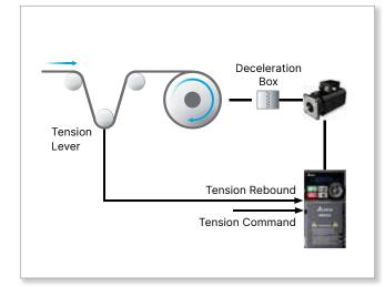
• Open-loop tension, torque control
