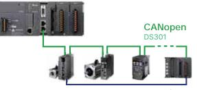
Supports up to 8 servo drives, 8 AC motor drives, and 7 AS RIO stations
