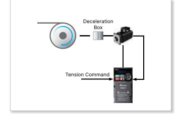
• Closed-loop tension, torque control
