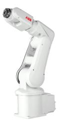
The IRB 120 robot is the latest addition to ABB's new fourthgeneration of robotic technology. It is ideal for material handling and assembly applications and provides an agile, compact and lightweight solution with superior control and path accuracy.
