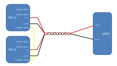
Fig. 29: Parallel connection without remote sense
