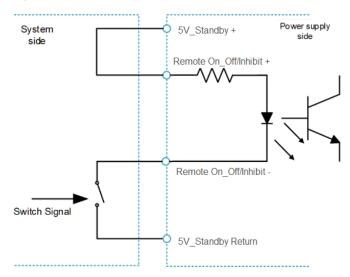
Fig. 24: Remote On\_off connection
