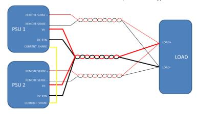
Fig. 28: Parallel connection with remote sense
