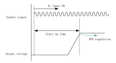
Fig. 18: Start-up timing sequence
