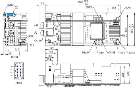
Fig. 7: Dimensional drawing Triple Slot Module
