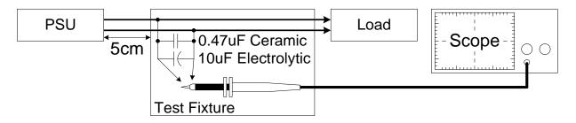
Fig. 22: Ripple and noise measurement circuit
