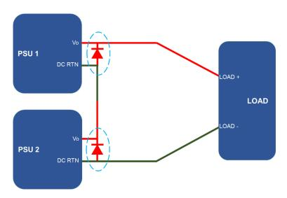
Fig. 30: Series connection with external reversed diode
