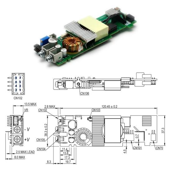
Fig. 6: Dimensional drawing Single Slot Module
