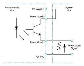
Fig. 25: Power good signal connection
