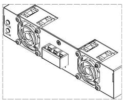
Figure 9. IEC320-C22 CONDUCTOR SIZE: 12-14 AWG
