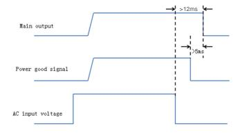
Fig. 26: Power good signal sequence
