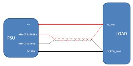
Fig. 27: Remote sense connection
