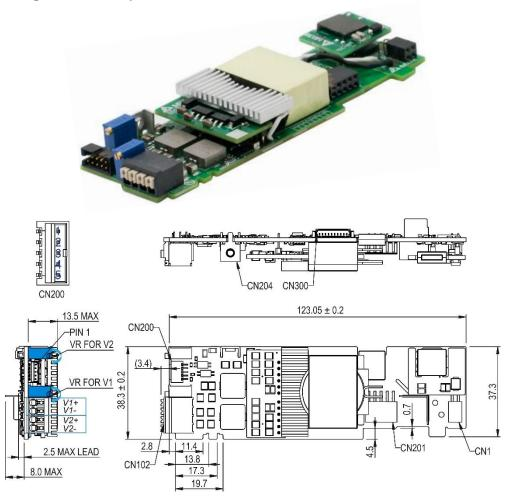
Fig. 8: Dimensional drawing Single Slot Dual Output Module
