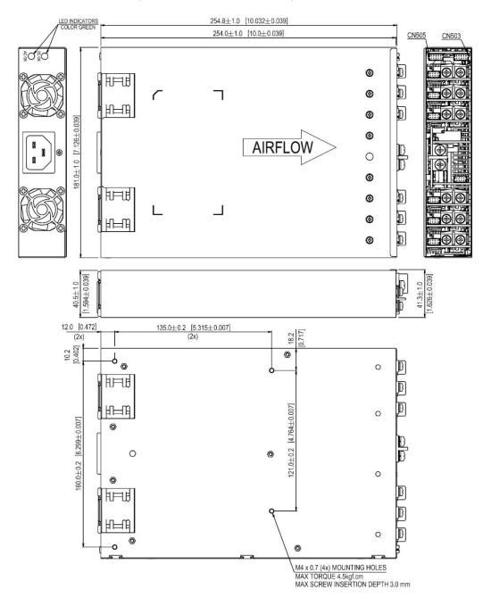
Fig. 5: Dimensional drawing MEG-3K0A
