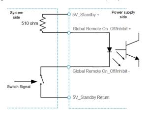
Fig. 31: Global Remote On\_off connection
