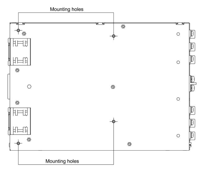
Fig. 4: Position of mounting holes
