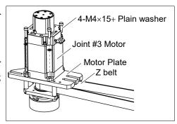
(10) Loosen the screws of the pulley remove it from the Joint #3 motor.
