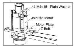
(3) Loosely secure the Joint #3 motor unit to the Arm #2. Make sure that the teeth of the timing belt are engaged with those of the pulley.
