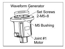
(9) Remove the motor mounting screws, and then remove the motor flange and O-ring.
