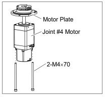
Joint #4 motor Installation (1) Mount the Joint #4 motor on the motor plate.
