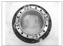
(6) Set the O-ring removed in the removal step (6) into the O-ring groove of the Arm #1.
