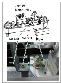
(7)-3 Check the tension using the sonic tension meter.
