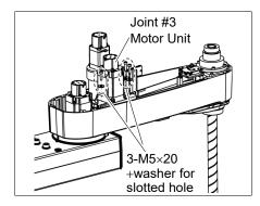
(5) Mount the User Plate and the Duct Plate.
