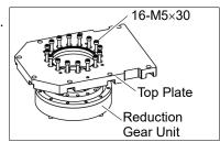
Joint #1 Reduction Gear Unit Installation
