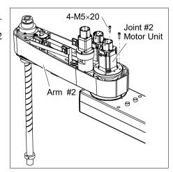
(5) Mount the User Plate and Duct Plate.
