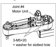
If the unit is tilted, the belt will not have the proper tension.
