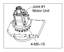
(4) Mount the Joint #1 unit on the Base.
