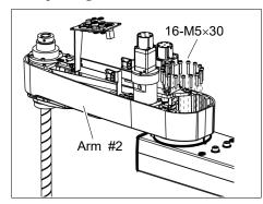
(6) Remove the reduction gear unit from the Arm #1 by removing the screws that mounts the reduction gear unit on the Arm #1.
