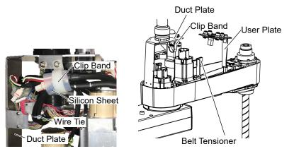
(6) Remove the Duct Plate.
