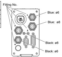
(4) Connect two connectors on the Base side.
