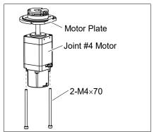
(15) Remove the brake from the motor plate.
