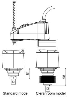
The height of Joint #3 depends on manipulator model.
