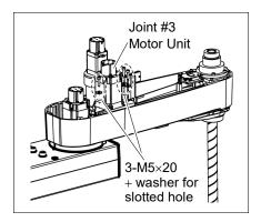
(8) Remove the Joint #3 motor from the motor plate.
