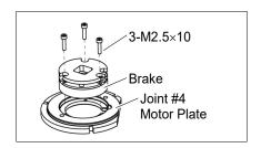
Joint #4 Brake Installation
