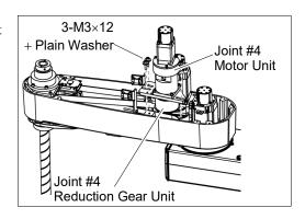
(10) Remove the screws mounting the spline plate.
