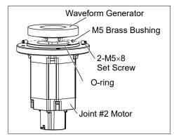
(10) Remove the motor flange from the Joint #2 motor.
