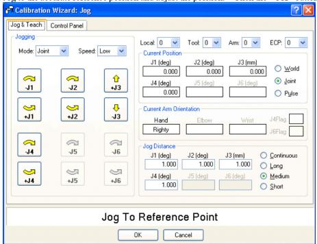
iii. Jog to the accurate reference position and adjust the position. Click the <OK> button.
