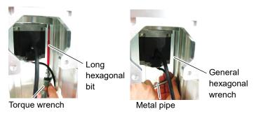
After loosening the screws, rotate the motor to pull out. If the motor is hard to pull out, pull the motor while rotating the Arm #1 slowly.
