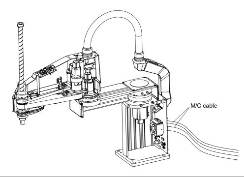
■ If the connectors have been disconnected during the replacement of the cable unit, be sure to reconnect the following connectors to their proper positions. Refer to the block diagrams. Improper connection of the connectors may result in improper function of the robot system.
