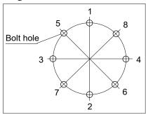
Do not fasten all bolts securely at one time. Divide the number of times that the bolts are fastened into two or three and fasten the bolts securely with a hexagonal wrench. Then, use a torque wrench so that the bolts are fastened with tightening torques shown in the table above.
