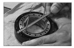
(5) Secure the cross roller bearing to the circular spline.
