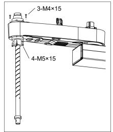
(9) Remove four screws mounting the spline nut.
