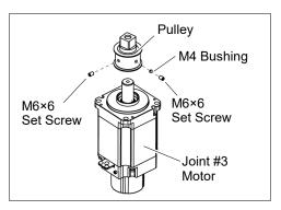
Joint #3 motor Installation (1) Mount the pulley to the Joint #3 motor.
