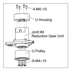
(3) Mount the Joint #4 motor unit on the reduction gear unit.
