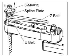
(2) Hold up the spline plate and set the Z belt around the Z pulley. Make sure the teeth of the timing belt are engaged with those of the pulley.
