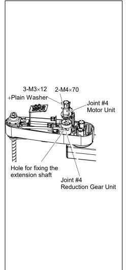
(10) Check if the Joint #4 moves in a Jog motion by operating from EPSON RC+ menu - [Tools]-[Robot Manager]-[Jog & Teach].
