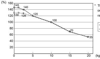
The percentage in the graph is based on the acceleration/ deceleration at rated weight (10 kg) as 100%.
