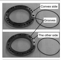
(3) Face the convex side of the circular spline down, and then fit it into the flexspline.
