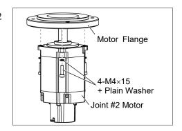
(2) Mount the waveform generator on the Joint #2 motor.
