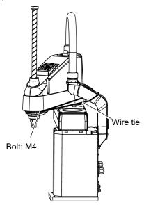
(3) Hold the bottom of Arm #1 by hand to unscrew the anchor bolts. Then, remove the Manipulator from the base table.
