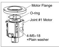
Joint #1 motor Installation (1) Put the O-ring on the motor mounting surface and mount the motor flange.
