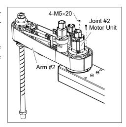
(9) Remove the waveform generator from the Joint #2 motor.
