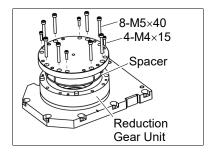
(3) Remove the reduction gear unit from the Top Plate.
