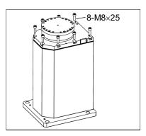
(7) Loosen the motor mounting screws on the motor flange and remove the motor unit
