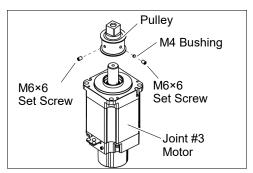
Tighten one of the set screws vertically on the flat face of the motor shaft. Insert a bushing into the other set screw hole to prevent damage to the motor shaft.
