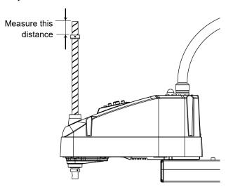
(6) Firmly tighten the lower limit mechanical stop screw (set screws: 2-M5×6).
