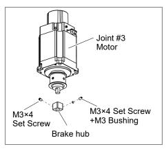
(3) Mount the Joint #3 motor to the motor plate while aligning the hub to the brake disc.
