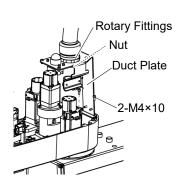
(17) Remove the rotary fitting from the metal duct.
