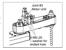
(9) Remove the Joint #3 motor from the motor plate and pull out the Z belt.
