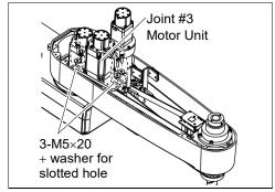
(9) Remove the Joint #3 motor from the Motor Plate.
