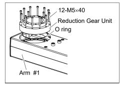
Joint #2 Reduction Gear Unit Installation
