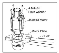
(5) Loosely secure the Joint #3 motor unit to the Arm #2.
