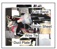
(8) Remove the screws mounting the motor unit and then remove the Joint #2 motor unit from the Arm #2.
