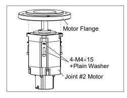
Joint #2 Motor Installation (1) Mount the motor flange on the Joint #2 motor.
