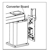
(4) Remove the converter board from the mount base.
