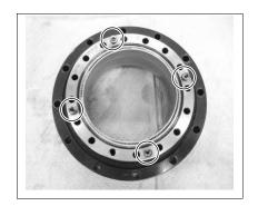
(6) Secure the Top Plate to the circular spline.
