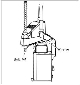
(3) Remove the screw for fixing the arm.
