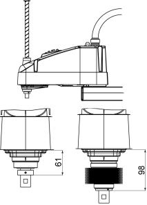
The height of Joint #3 depends on manipulator model.
