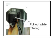
(8) Remove the waveform generator from the Joint #1 motor.
