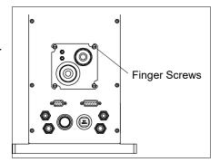
(4) Slide the plate to remove it from the base.
