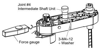
NOTE To check belt tension with the tension meter, refer to *Maintenance: 8.4 Checking the Timing Belt Tension (U1, U2 Belts).*
