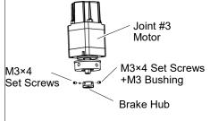
Joint #3 brake (1) Mount the brake to the brake plate. Installation
