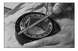
(5) Secure the reduction gear flange to the circular spline.
