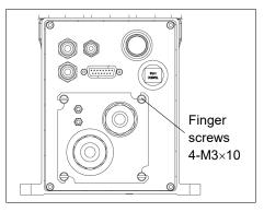
(4) Slide the plate to remove it from the base.
