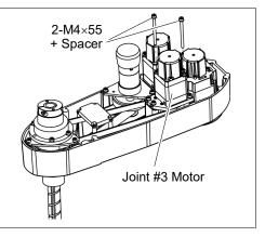
(10) Loosen the screws of the pulley and the brake hub. Remove them from the Joint #3 motor.
