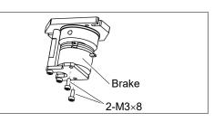
(2) Mount the brake hub to the pulley of the Joint #3 motor.
