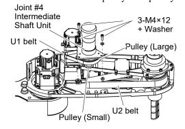
(2) Loosely secure the Joint #4 intermediate shaft unit.
