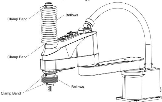
For the Cleanroom-model, the following parts are added to the Standard-model.
