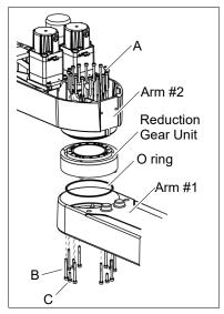
Joint #2 Reduction Gear Unit Installation  A new reduction gear unit contains the parts shown in the picture on the right when it is unpacked.
