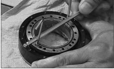
(5) Set the O-ring removed in the removal step (6) into the O-ring groove of the Arm #1.
