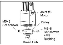
(1) Mount the pulley and the brake hub to the Joint #3 motor.
