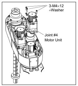
(5) Apply the proper tension to the U1 belt, and then secure the Joint #4 motor unit.
