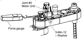
NOTE To check belt tension with the tension meter, refer to *Maintenance: 8.4 Checking the Timing Belt Tension (U1, U2 Belt).*
