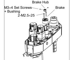
Joint #4 brake Installation
