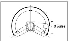
0 pulse position of Joint #2: position where Arms #1 and #2 are in a straight line (Regardless of the Joint #1 direction.)
