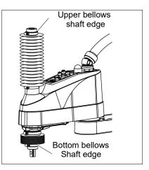
(5) When completed the bellows installation, check that the bellows stretch smoothly without any excessive force by moving the shaft up/down by hand and rotating the Joint #4.
