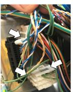
(8) Cut off the two wire ties binding the cables on the base side cable fixing plate.
