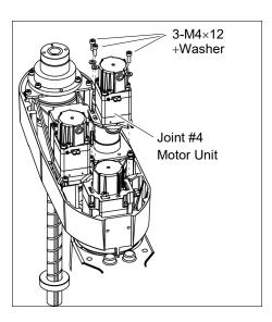
(2) Remove the Joint #4 intermediate shaft unit.
