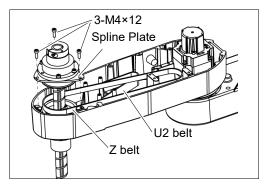
(10) Remove the screws securing the Joint #4 motor unit and pull out the motor unit.
