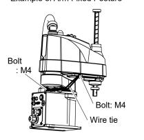
(3) Hold the bottom of Arm #1 by hand to unscrew the anchor bolts. Then, remove the Manipulator from the base table.
