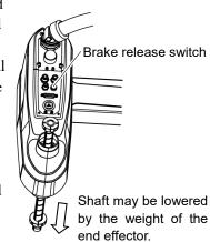
This button switch is a momentary-type; the brake is released only while the button switch is being pressed
