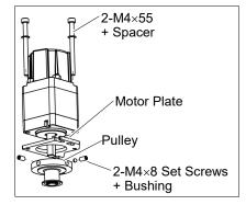
Be sure to fit the end face of the pulley to the end face of the motor shaft.
