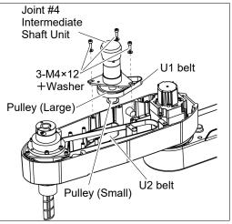
(5) Loosely secure the Joint #4 intermediate shaft unit.
