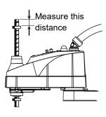
(6) Firmly tighten the lower limit mechanical stop screw (M4 $\times$ 15).
