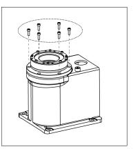
(6) Loosen the motor mounting screws on the Joint #1 motor flange and remove the motor unit
