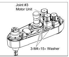
(9) Remove the Joint #3 motor from the Joint #3 motor unit.
