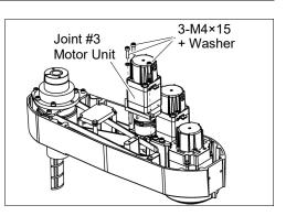
Apply the proper tension to the Z belt, and then secure the Joint #3 motor unit.
