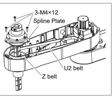
(2) Hold up the spline plate and set the Z belt around the Z2 pulley.
