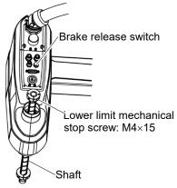
NOTE When you press the brake release switch, the shaft may lower due to the weight of the end effector. Be sure to hold the shaft by hand while pressing the button.
