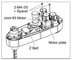
(3) Loosely secure the Joint #3 motor unit to the Arm #2. Make sure that the teeth of the timing belt are engaged with those of the pulley.
