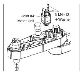
Make sure the motor unit can be moved by hand, and it will not tilt when pulled. If the unit is secured too loose or too tight, the belt will not have the proper tension. (9) Apply the proper tension to the U1 belt and secure the Joint #4 motor unit.
