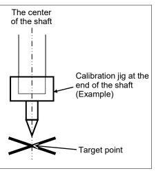
After removing the end effector and executing the calibration, install the end effector and move the Manipulator to the teaching point to verify whether there is a positional gap. If there is a positional gap, fine-tune the installation position of the end effector and teach the point again.
