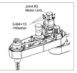
(12) Loosely secure the Joint #3 motor unit to Arm #2.
