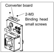
Converter board (1) Mount the converter board on the mount base. Installation Binding head small screws: (2-M3)
