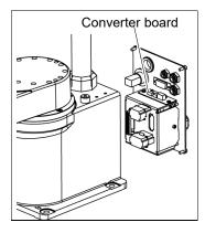
(4) Remove the converter board from the mount base.Binding head small screws:2-M3 (cross-point screwdriver)
