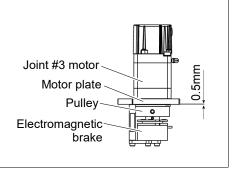
Tighten one of the set screws vertically on the flat face of the motor shaft.
