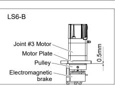
Tighten one of the set screws vertically on the flat face of the motor shaft. Insert a bushing into the other set screw hole to prevent damage to the motor shaft.
