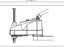
The height of Joint #3 (shaft) depends on manipulator model.
