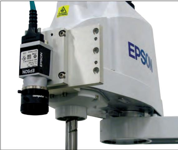
Synthesis T-Series shown with mobile mounted camera as part of the Epson Vision Guide option
