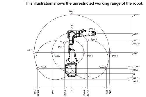
Positions at wrist center and angle of axes 2 and 3
