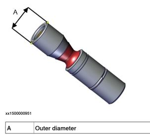
Periodic check of the calibration tool for the tool flange (3HAC058238-001)
