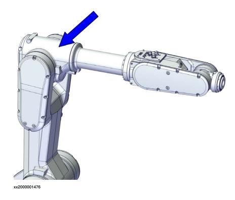
The extender unit (only for IRB 1300-7/1.4 and IRB 1300-12/1.4) is located as shown in the figure.
