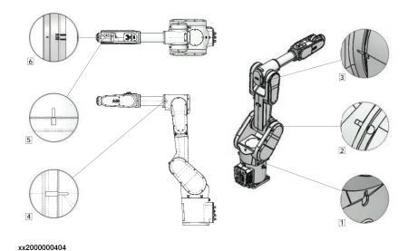
6.2.2 Calibration movement directions for all axes
