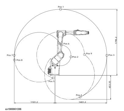
Positions at wrist center and angle of axes 2 and 3
