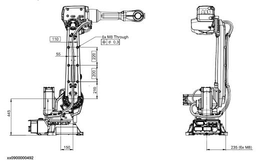
The uppermost holes for fitting equipment on the lower arm are only applicable to variant IRB 2600 -12/1.85.
