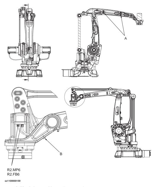
The motor axis 6 is located as shown in the figure below.
