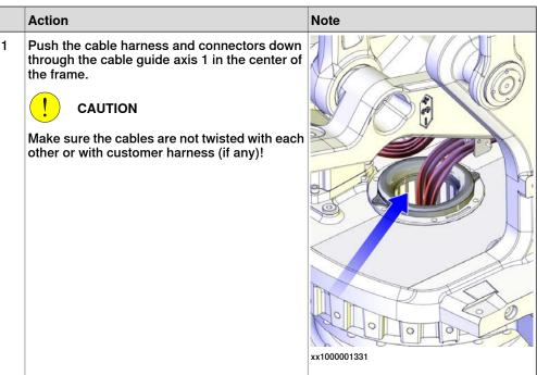
4.3.1 Replacing cable harness, lower end (axes 1-3) *Continued*
