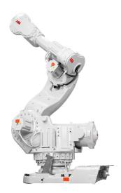
With several variants, and up to a 630 kg handling capacity, the IRB 7600 is ideal for weighty applications, regardless of your industry. Characteristics such as high available torque and inertia capability, rigid design, and powerful acceleration have earned this market leader its "Power Robot" title.
