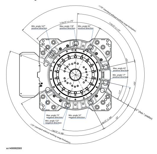
2.4.2 Mechanically restricting the working range of axis 1
