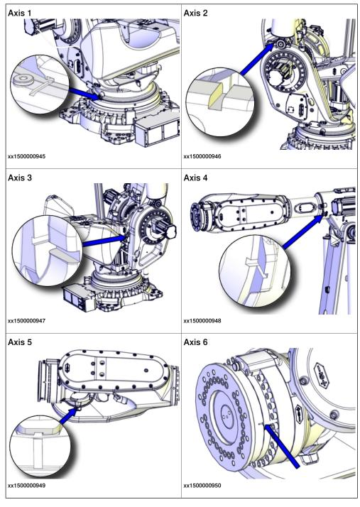
5.2.2 Calibration movement directions for all axes
