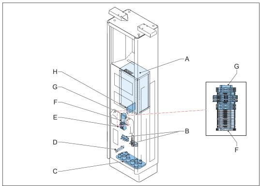
Cooling unit Α Ε Q1 RCD В DC power busbars F X-10 terminal block С Cable gland plates G X-20 terminal block D PE busbar CAN2FIBER device Н
