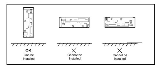
Fig. 2.9 Driver Installation Direction
