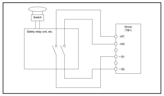
Fig. 3.22 Wiring Example of Safety Function Terminal
