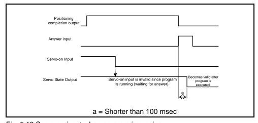
Fig. 5.13 Servo-on input when program is running
