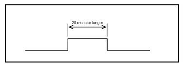
Fig. 5.1 Input Signal ON-time
