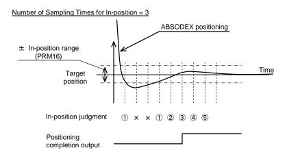
Fig. 7.6 Position Completion Output
