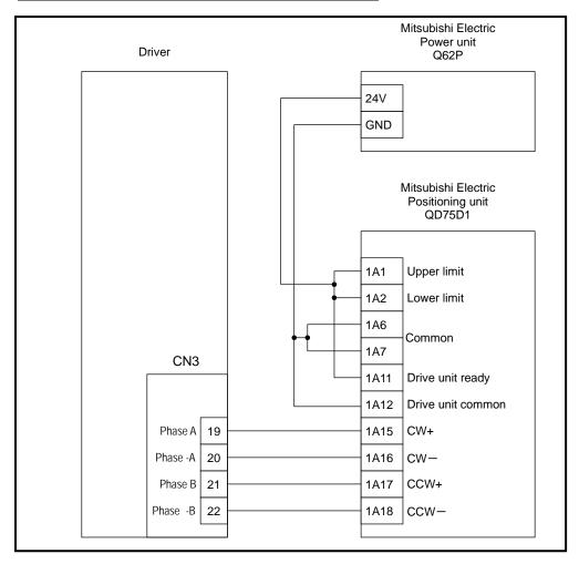
Fig. 3.20 Wiring Example of System Operating with Pulse String Inputs
