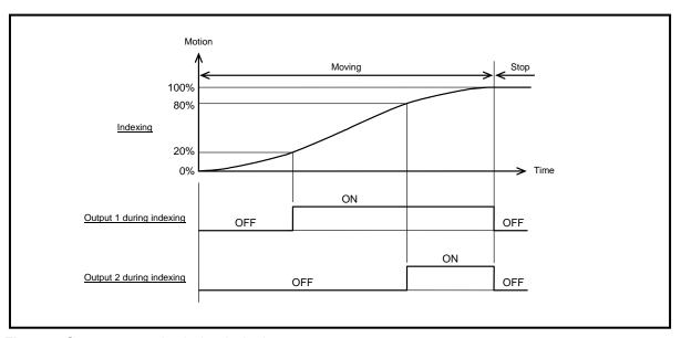
Fig. 518 Output example during indexing (In case of PRM33 = 20, PRM34 = 80)
