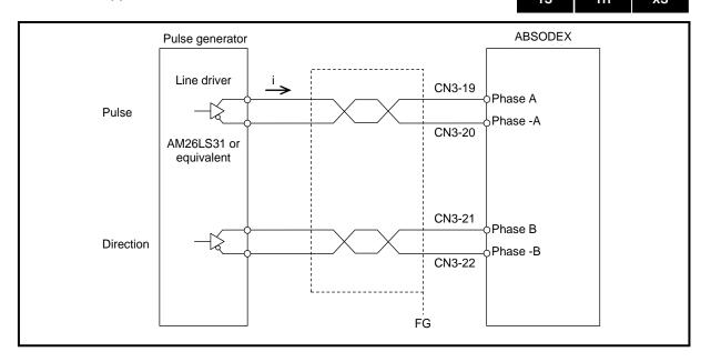
Fig. 3.17 Connection Example 2 of Pulse String Input
