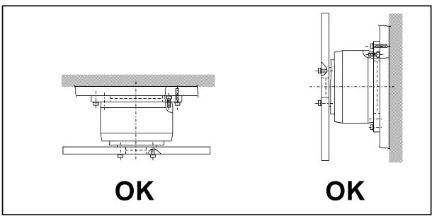
Fig. 2.6 Direction of Installation of Actuator
