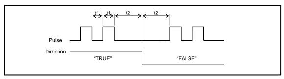
Fig. 5.21 Pulse & Direction Inputs
