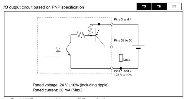
Fig. 3.15 I/O output circuit based on PNP specification
