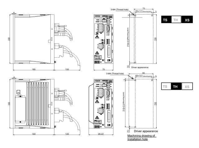
Fig. 2.10 Dimensions of Driver (Figure above: TS Type Driver and XS Type Driver, Figure below: TH Type Driver)
