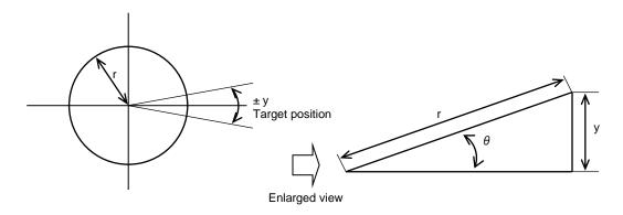
Fig. 7.7 Correct In-position Range
