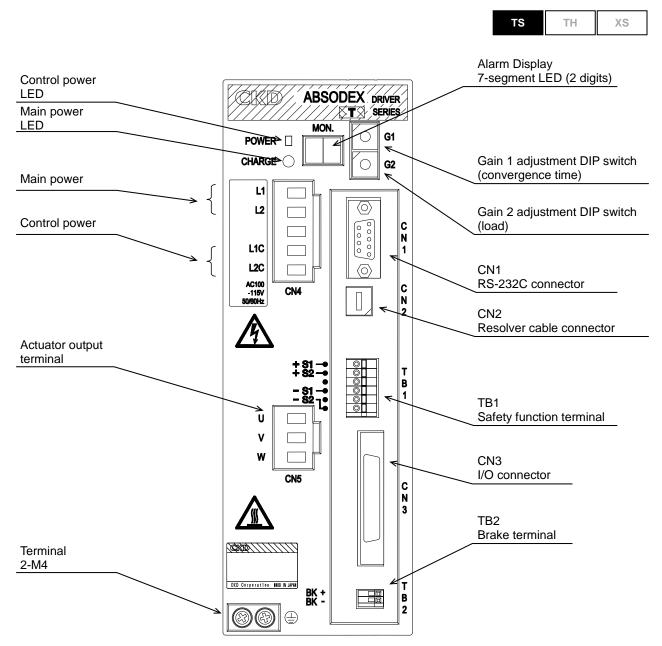
Fig. 3.4 TS Type Driver Panel 100 VAC specification
