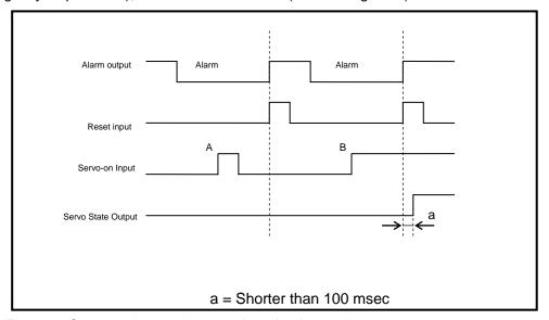
Fig. 5.12 Servo-on input when an alarm is triggered
