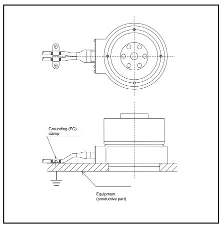
Fig. 16.4 Grounding Example on Actuator Side
