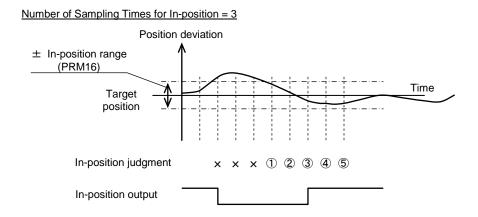
Fig. 7.5 In-position Output
