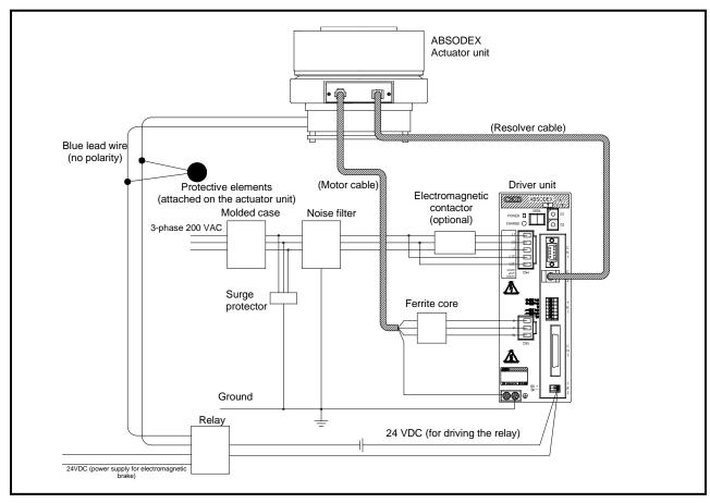
Fig. 3.23 Wiring the Electromagnetic Brake
