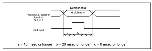
Fig. 5.8 Timing of Program Number Input
