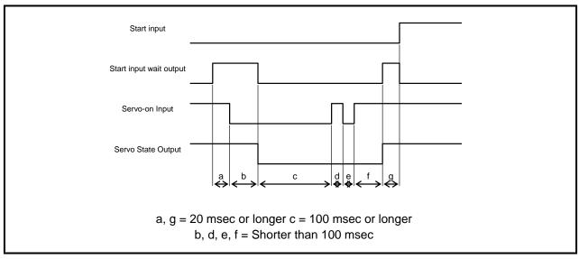
Fig. 5.11 Timing Chart of Servo-on Input
