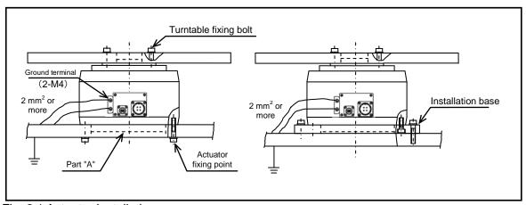
Fig. 2.1 Actuator Installation
