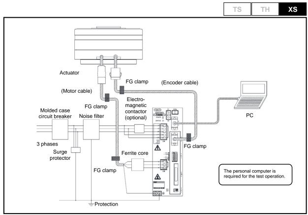
Fig. 4.3 Connection Example of XS Type Driver (3-Phase 200 VAC Power Supply)
