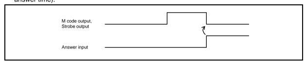
Fig. 5.17 M Code Output Timing
