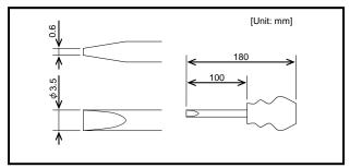
Fig. 3.9 Dimensional Drawing of Recommended Regular Screwdriver
