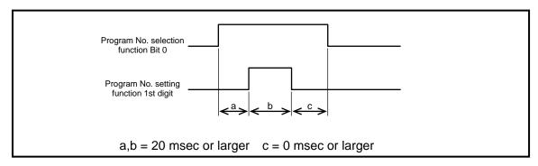
Fig. 5.5 Timing of Program Number Input
