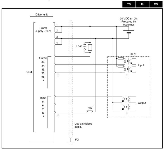
Fig. 3.10 Connection based on NPN specification (example)
