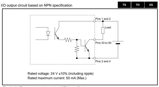
Fig. 3.13 I/O output circuit based on NPN specification
