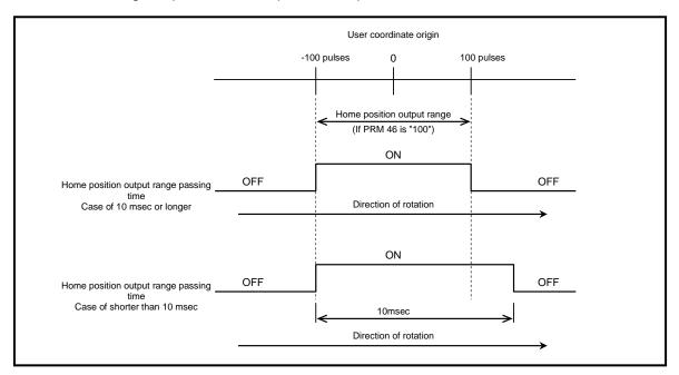
Fig. 5.19 Home Position Output Timing
