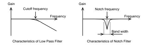
Fig. 7.9 Filter Characteristics
