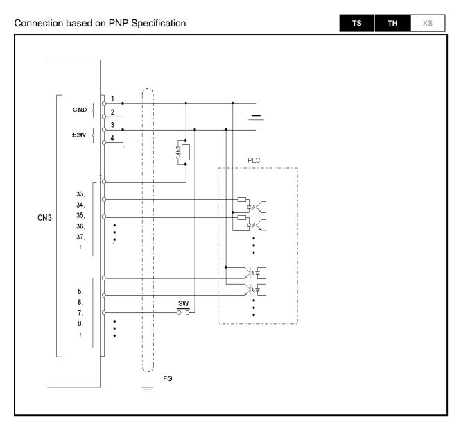
Fig. 3.11 Connection based on PNP specification (example)
