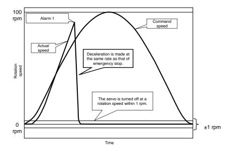
Fig. 7.12 Example of Speed Curve at Alarm
