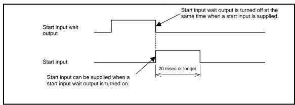
Fig. 5.9 Start Input Timing
