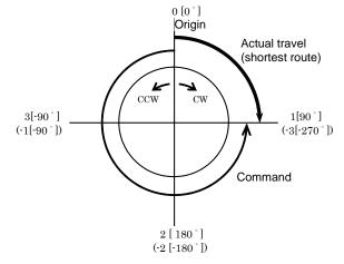
The upper stage indicates the actual travelling angle [indexed count], and the lower stage indicates the designated angle [indexed count] in the command.
