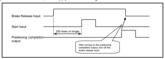
Fig. 5.10 Timing of Brake Release Input
