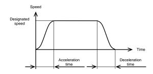
If the traveling time determined by the angle of travel and designated speed is equal to the sum of the acceleration time and deceleration time, the constant velocity interval is eliminated.
