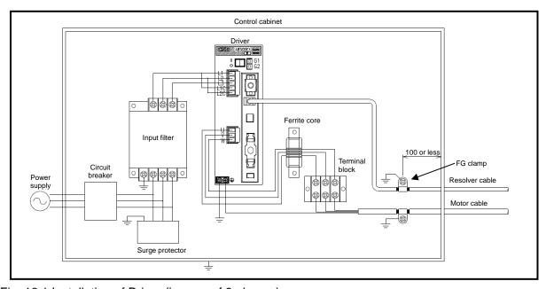
Fig. 16.1 Installation of Driver (in case of 3 phases)
