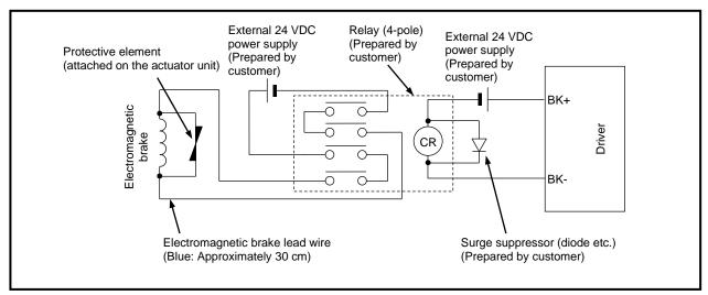
Fig. 3.25 Recommended Circuit 2 for Electromagnetic Brake
