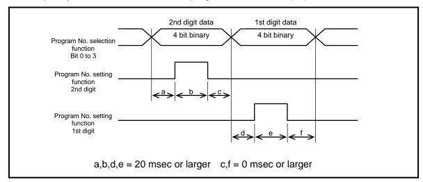
Fig. 5.3 Timing of Program Number Input
