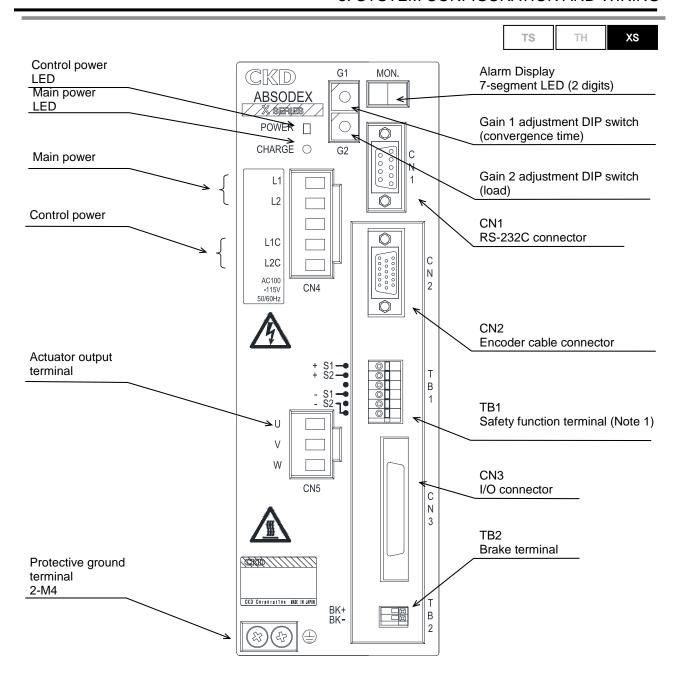
Fig. 3.7 XS Type Driver Panel 100 VAC specification
