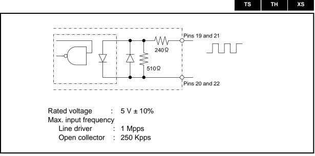
Fig. 3.18 Pulse String Input Circuit
