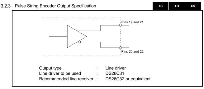
Fig. 3.19 Encoder Output Circuit
