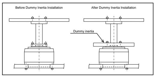
Fig. 2.3 Dummy Inertia Installation 1
