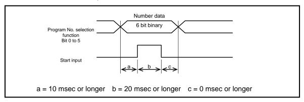
Fig. 5.7 Timing of Program Number Input
