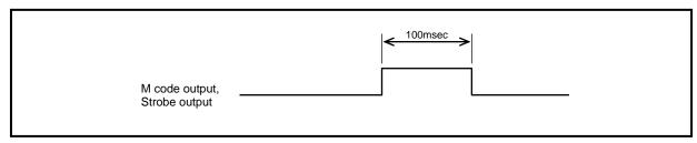
Fig. 5.16 M Code Output Timing
