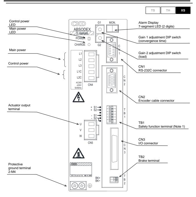
Fig. 3.6 XS Type Driver Panel 200 VAC specification
