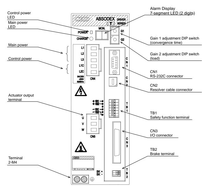
Fig. 3.3 TS Type Driver Panel 200 VAC specification
