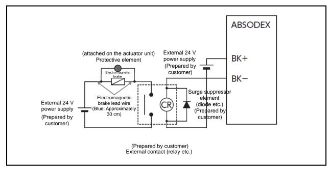
Fig. 3.24 Recommended Circuit 1 for Electromagnetic Brake
