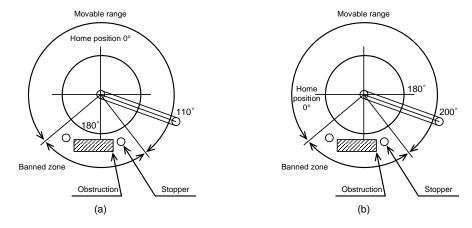
Fig. 8.6 Coordinate System Setting
