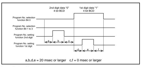
Fig. 5.6 Timing of Program Number Input
