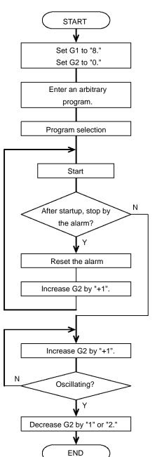
Use a regular screwdriver or the like to change gain adjustment DIP switches G1 at "8" and G2 at "0" on the driver panel.
