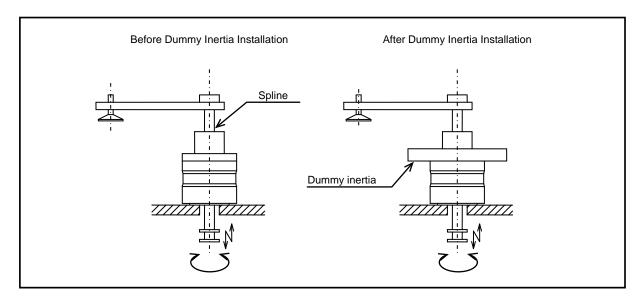
Fig. 2.5 Dummy Inertia Installation 3
