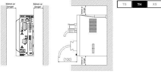
Fig. 2.8 TH Driver Installation Interval
