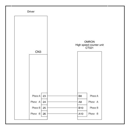
Fig. 3.21 Wiring Example of System Operating with Encoder Outputs
