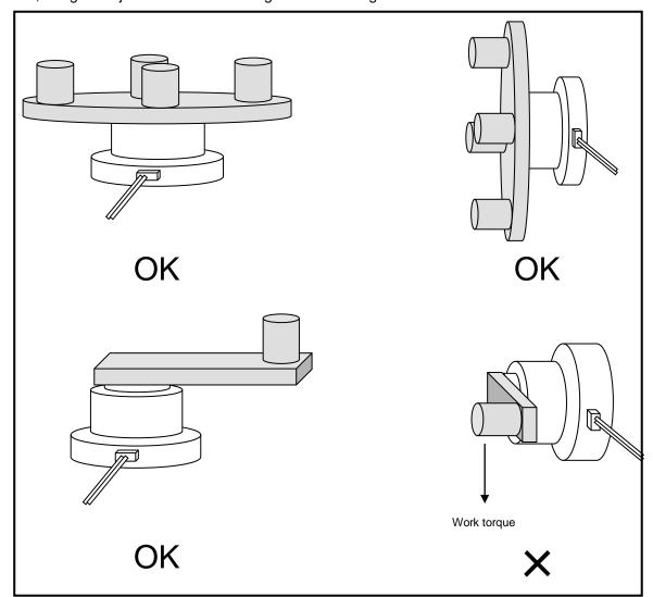
Fig. 4.4 Action of Work Torque
