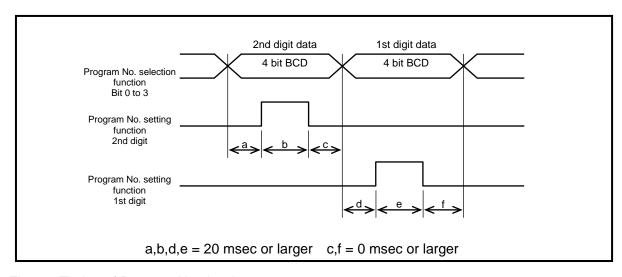
Fig. 5.2 Timing of Program Number Input
