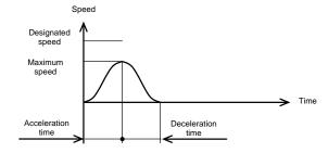
The acceleration time and deceleration time are specified in PRM 2.
