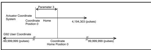
Fig. 6.1 ABSODEX Coordinate System
