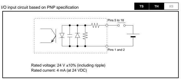
Fig. 3.14 I/O input circuit based on PNP specification
