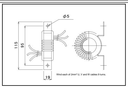
Fig. 16.3 Ferrite Core 1
