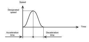
Further, if the traveling time is shorter than the sum of the acceleration time and deceleration time, the traveling time is corrected to the sum of the acceleration time and deceleration time, and the maximum speed is reduced.
