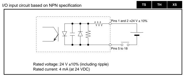
Fig. 3.12 I/O input circuit based on NPN specification
