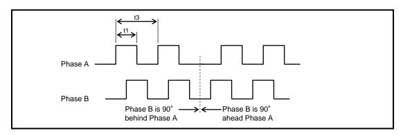
Fig. 5.23 A and B Phase Inputs
