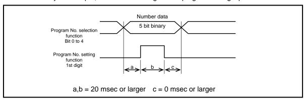
Fig. 5.4 Timing of Program Number Input
