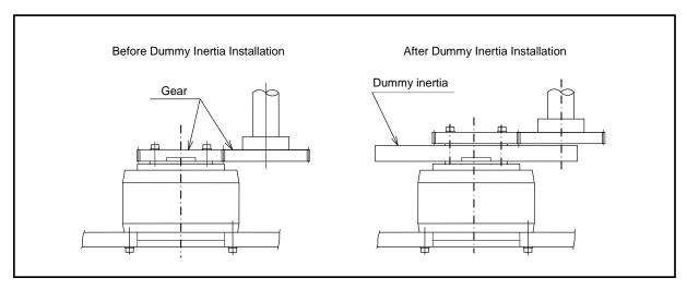
Fig. 2.4 Dummy Inertia Installation 2
