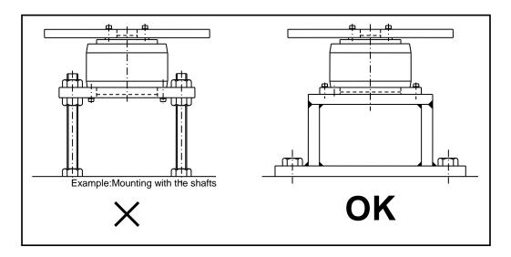
Fig. 2.2 Actuator Installation Method
