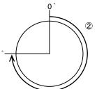
If the rotation speed is high and the traveling amount is smaller, the acceleration may become too large to cause alarm 1 (position deviation over).
