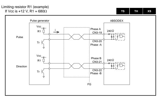
Fig. 3.16 Connection Example 1 of Pulse String Input
