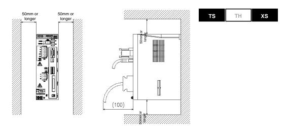
Fig. 2.7 TS Type Driver/XS Type Driver Installation Interval
