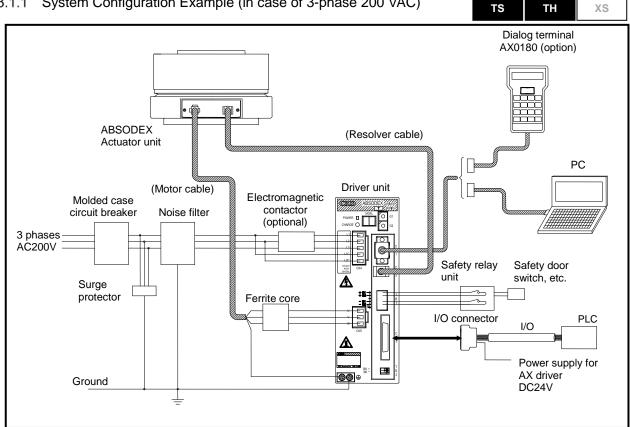
Fig. 3.1 System Configuration (TS Type Driver/TH Type Driver)
