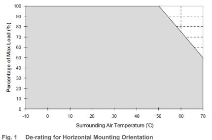
**De-rating for Horizontal Mounting Orientation** > 50°C de-rate power by 2.5% / °C
