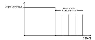
It is not recommended to prolong the duration of  $I_{\rm O}$  when it is <125% but >100%, since it may cause damage to the PSU.
