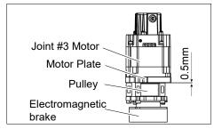
Tighten one of the set screws vertically on the flat face of the motor shaft. Insert a bushing into the other set screw hole to prevent damage to the motor shaft.
