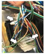
(8) Cut off the two wire ties binding the cables on the base side cable fixing plate.
