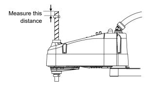
(6) Firmly tighten the lower limit mechanical stop screw (set screws: 2-M5×6).
