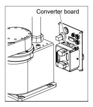
(4) Remove the converter board from the mount base. Binding head small screws:
