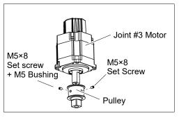
Joint #3 motor Installation
