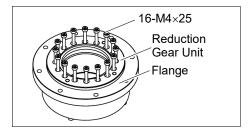
Joint #1 Reduction Gear Unit Installation
