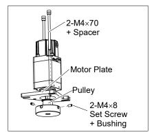
Be sure to fit the end face of the pulley to the end face of the motor shaft.
