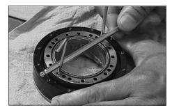
(5) Set the O-ring removed in the removal step (6) into the O-ring groove of the Arm #1.
