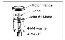
Joint #1 motor Installation (1) Set the O-ring (CO0538A) on the motor mounting surface and mount the motor flange.
