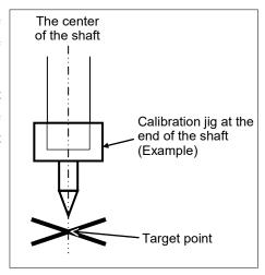
After removing the end effector and executing the calibration, install the end effector and move the Manipulator to the teaching point to verify whether there is a positional gap. If there is a positional gap, fine-tune the installation position of the end effector and teach the point again.
