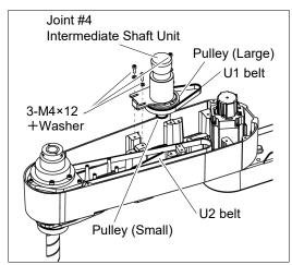
(5) Loosely secure the Joint #4 intermediate shaft unit.
