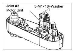
(6) Remove the Joint #3 motor from the Joint #3 motor unit. The belt is placed around the pulley. To remove the Joint #3 motor, tilt the motor slightly and pull it upward while avoiding the belt.
