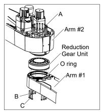
Loosely secure all bolts in a crisscross pattern so that the bolts will be secured evenly. Then, using a torque wrench, tighten each bolt securely in a crisscross pattern at the torque specified in the table below.
