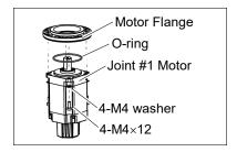
(2) Apply grease (SK-1A) to the between the waveform generator and motor.
