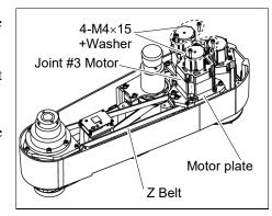
(3) Loosely secure the Joint #3 motor unit to the Arm #2. Make sure that the teeth of the timing belt are engaged with those of the pulley.
