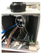
(9) Remove the seven ground wires that secured on the mount base.
