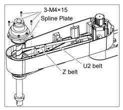
(2) Hold up the spline plate and set the Z belt around the Z2 pulley.Make sure the gear grooves of the belt are fit into those of the pulleys completely.
