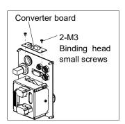
(2) Connect the connectors to the converter board.
