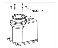
(6) Loosen the motor mounting screws on the Joint #1 motor flange and remove the motor unit
