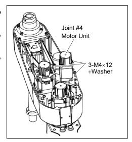
(5) Apply the proper tension to the U1 belt, and then secure the Joint #4 intermediate shaft unit.
