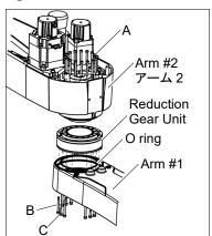
Joint #2 Reduction Gear Unit Installation
