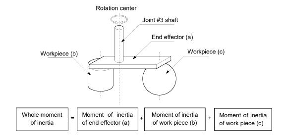
The methods for calculating the moment of inertia for (a), (b), and (c) are shown below. Calculate the total moment of inertia using the basic formulas.
