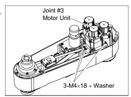
(9) Remove the Joint #3 motor from the Joint #3 motor unit.
