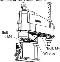
(3) Hold the bottom of Arm #1 by hand to unscrew the anchor bolts. Then, remove the Manipulator from the base table.
