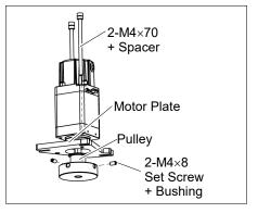
Joint #4 motor Installation
