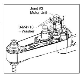
(12) Loosely secure the Joint #3 motor unit to Arm #2.
