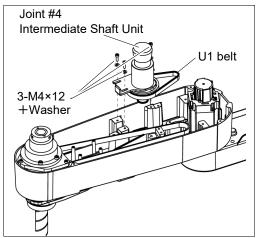
(12) Remove the screws mounting the spline plate.
