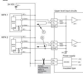
Note 1) Connecting more than one analog output 4-20 mA sensor to the same common input circuit (upper level computer, sequencer, etc.) as shown above makes the respective signals interfere with each other, preventing correct operation. In this case please use the voltage output type (standard, A2, A3).
