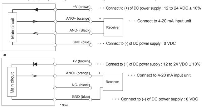
When connecting two or more flow rate sensors to the upper-level input circuit (receiver), carefully prevent signal interference.
